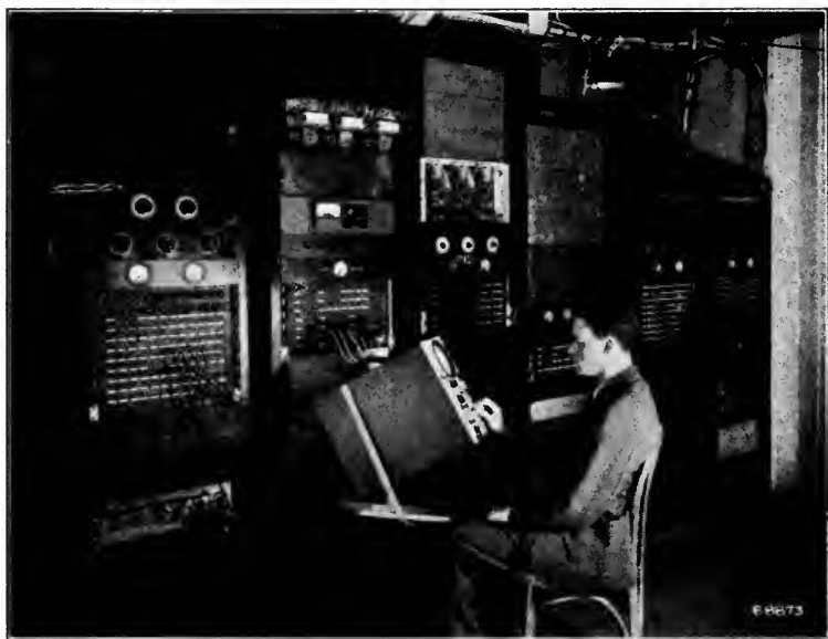
FIG. 1. Recording amplifiers, low-level reproducing amplifiers, and equipment for compressing and expanding the volume range.
